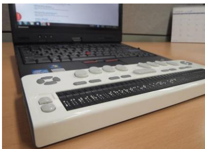
Figure 6 Braille Display Connected to a Laptop (retrieved from http://www.hims-inc.com/product/braille-edge-40/ )
